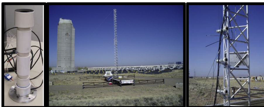
Fig. 1. Left: collimated LI-COR pyranometer. Middle: photo of trailer-mounted mobile heliostat target with NSTTF central receiver tower in background. Right: close-up of collimated pyranometers mounted on aluminum tower.
