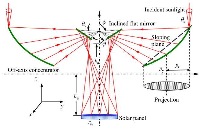
Fig. 1. Schematic of the principle of STFC.
