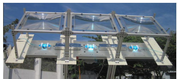
Fig. 2. A picture of a partially assembled collector frame mounted on a tracker showing Fresnel lenses focusing light on a volumetric absorber.
