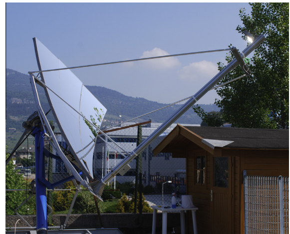
Fig. 1. Solar collector composed by three parabolic modules mounted on the sun tracking system.
