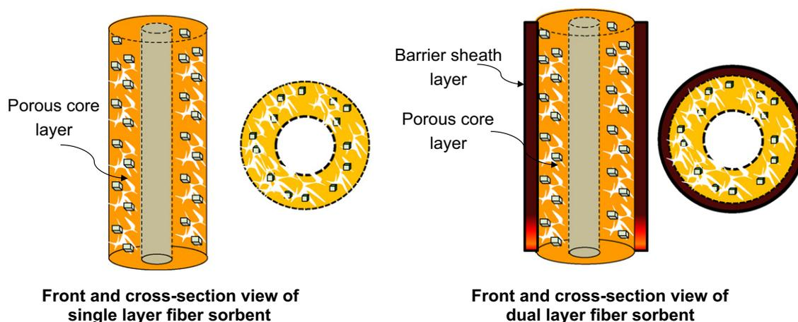
Fig. 1. Schematic diagram showing the key features of a single and dual layer hollow fiber sorbent.
