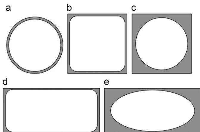
**Fig. 1.** Scheme of the liquid film distribution around gas bubbles in microchannel with different cross sections. (a) Circular channel, (b) square channel under transitional  $Ca$ , (c) square channel above transitional  $Ca$ , (d) and (e) rectangular channel.
