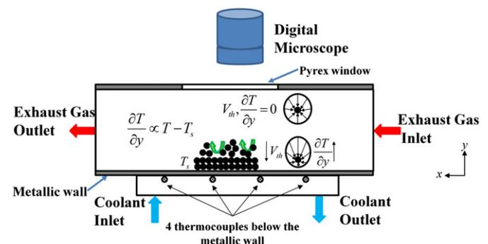
Fig. 2. Principle of the visualization test rig (side view)—metallic channel carries exhaust (or compressed air) and glass window allows visualization.
