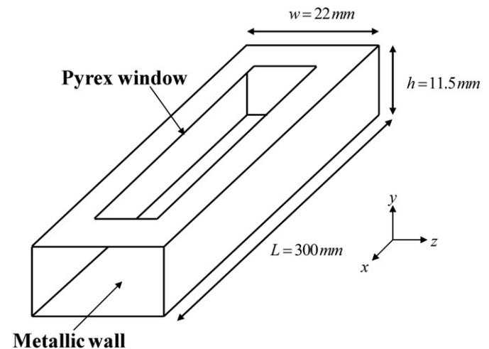
Fig. 1. Schematic of the channel (isometric view).
