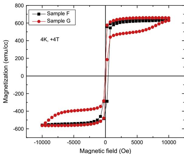
**Fig. 1.** Comparison of isothermal (4 K) magnetization reversal processes of sample F and sample G. This data were resulted after the samples were field cooled under +4T. Here, we kept the SRO layer thickness constant at 45 nm. As it can be seen, the magnetization reversal processes are distinctly different. Another notable observation is that a positive exchange bias (shift of hysteresis loop toward field cooled direction) is observed only for the former sample.
