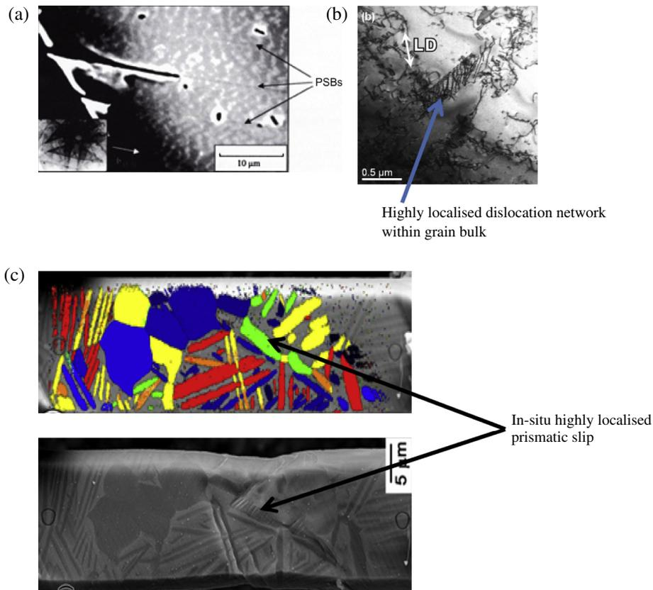
**Fig. 2.** (a) PSB and fatigue crack nucleation within single-crystal copper [2]; (b) dislocation structure within a grain in polycrystalline 316 steel [3] and (c) localised prismatic slip in a titanium alloy [5].
