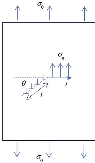
**Fig. 1.** Schematic diagram of the Stroh crack nucleation model showing a PSB of length  $l$ , orientated to a remote stress and in an infinite elastic medium.
