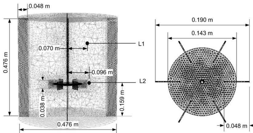
Fig. 1. Schematic presentation and computational grid of the stirred tank reactor with Rushton turbine (Left: Tank; Right: Impeller details).
