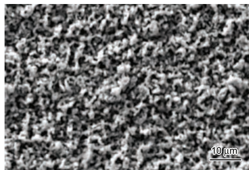
Fig. 1 SEM image of phosphorous black nickel coating
