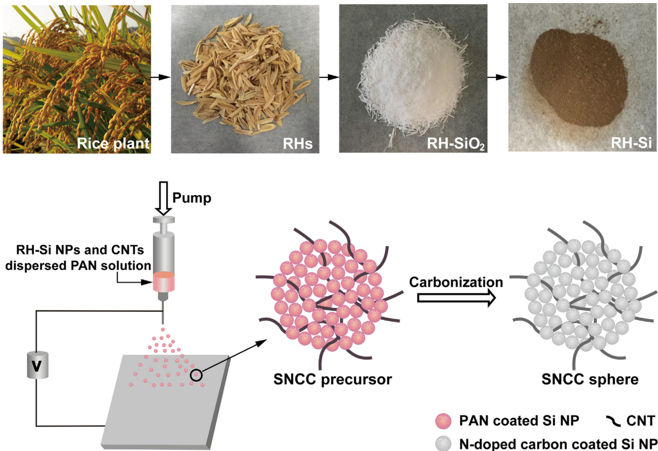
Fig. 1. Schematic illustration of the preparation process for SNCC nano/micro-structured spheres.
