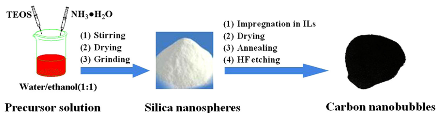
Scheme 1 Illustration for synthesis of silica nanospheres template and the carbon nanobubbles.
