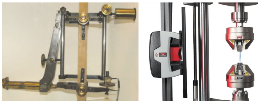
Fig. 1. Extensometers ancient and modern. (left) one of the earliest contacting extensometers produced by J. A. Ewing in Cambridge, c1890; (right) Instron AVE2 video extensometer for dynamic measurement, released 2015.
