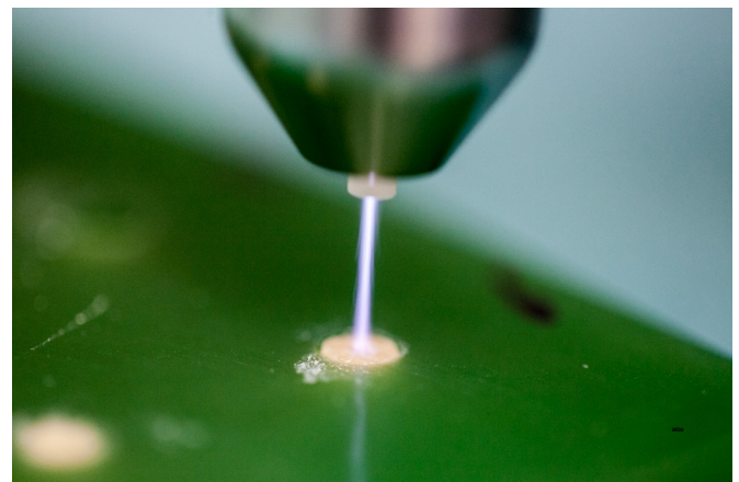
Fig. 1. Surface plasma irradiation of porcine bone cylinder.
