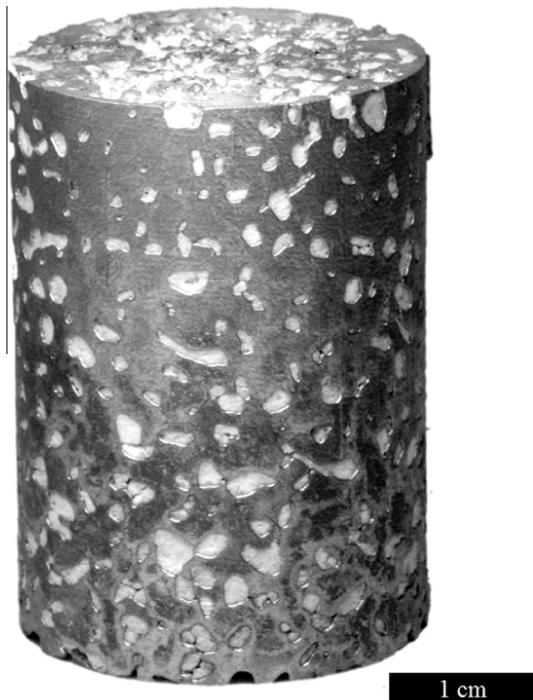
Fig. 1. Photograph of A356/perlite metallic syntactic material.
