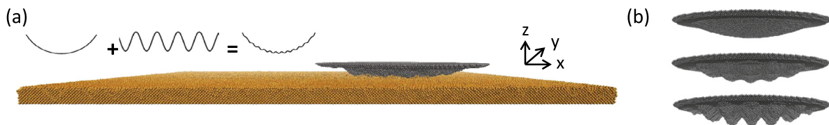
Fig. 1. (a) Snapshot of the simulation system consisting of a Si tip and Cu substrate during sliding. The inset shows the geometry of a rough tip created by superposing a spherical cap with a cosine wave. (b) Snapshots of a few of the model tips with different roughness: R_q = 0.184, 0.352 and 0.638 nm, from the top to the bottom image. Cu atoms are shown in orange, Si atoms in gray.
