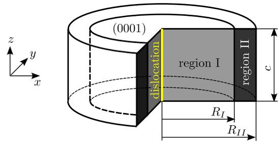
**Fig. 1.** A cylindrical simulation block used for the calculations in this paper. Periodic boundary conditions are applied along the  $z$  direction to study straight threading dislocations in the bulk.
