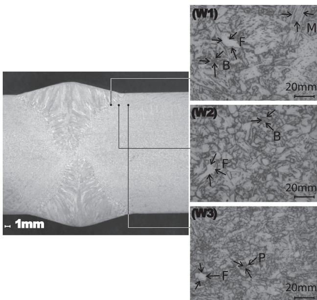
Fig. 1. Butt welded joint (DHY) and microstructure in particular regions of HAZ.
