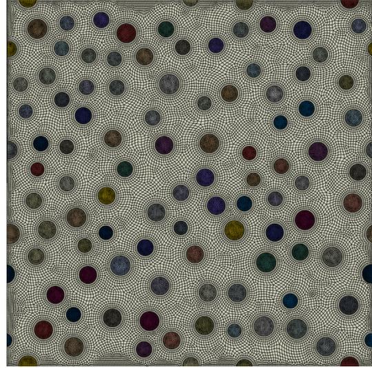
Fig. 1. Example of FE-mesh of microstructural model.
