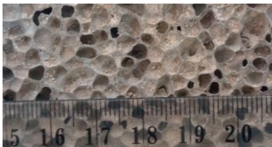
(a) Aluminium foam with a porosity of 88%
