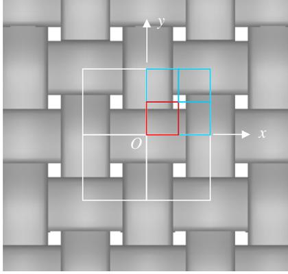
Fig. 1. Plain weave and unit cell models based on the use of various symmetries.
