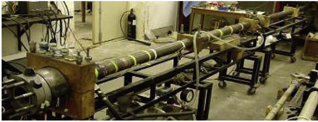
Fig. 1. The 63 mm bore gas gun used in the experiments. The test was carried out in a vacuum chamber to avoid compressed air between the target and impact face of the projectile.
