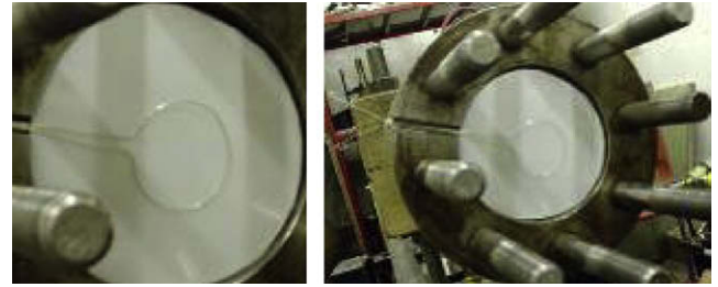
Fig. 3. Plastic bursting discs with wire heating loop mounted between them. The disc was held by two flanges which were attaching the barrel to the gas reservoir.
