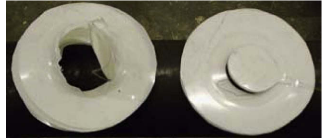
Fig. 4. Two examples of burst discs. The rupture of the discs with maximum four discs (pressure up to 7 MPa) was generally sharp cut but for more discs the rupture was not regular.
