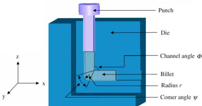
Fig. 1. Schematic diagram of an ECAP die channel angle  $\phi$  and the corner angle  $\psi$ .
