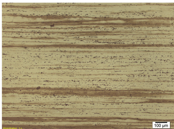
Fig. 1. Optical micrograph of as-extruded sample showing dark bands along extrusion axis (horizontal).
