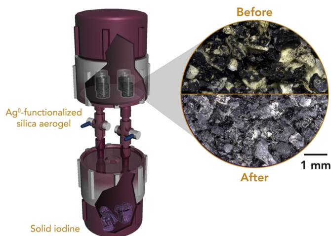
Fig. 1. Assembly to produce iodine-loaded \text{Ag}^0 -aerogel; samples were exposed to iodine vapors at 150^\circ\text{C} for 24 h.
