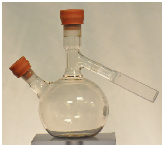
Fig. 1. Glass reactor made for radiolysis experiments. The reaction solution is deaerated by bubbling Ar into the vessel through a heavy gauge needle in the top stopper, while air and excess Ar are allowed to escape through a needle in a secondary stopper. Both needles are removed prior to radiolysis.
