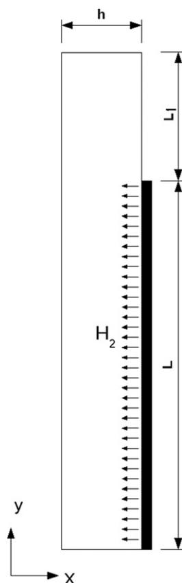
Fig. 1. The single channel geometry used in the simulations (figure not in scale).
