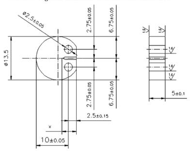
Fig. 1. Schematic representation of the disc-shaped in tension (DCT) specimen; dimensions in mm.
