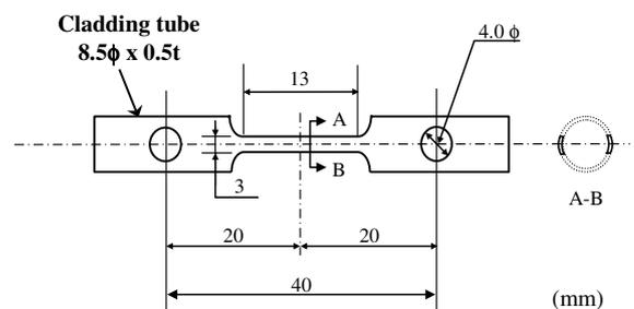
Fig. 1. The specimen dimensions.
