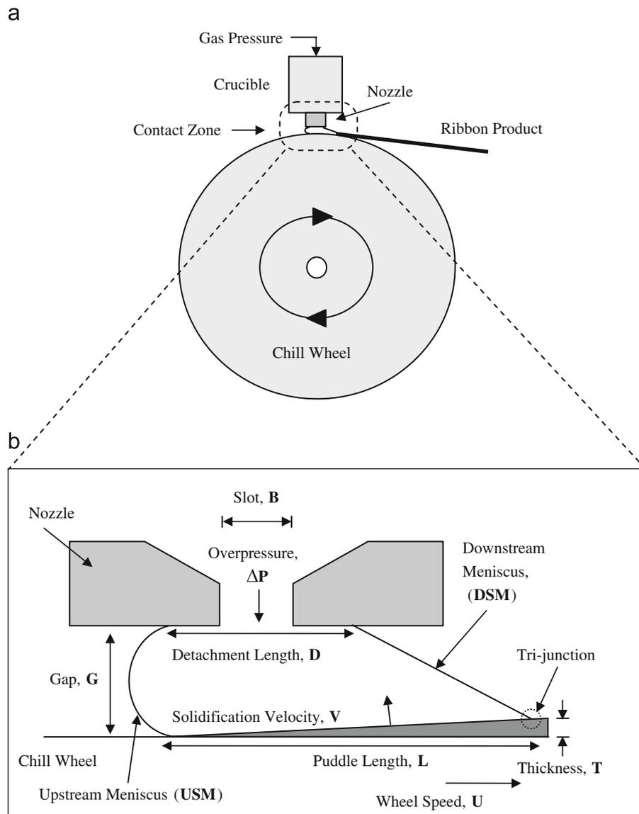
**Fig. 1.** (a) Schematic of the PFMS apparatus. Molten metal flows from the crucible through a nozzle onto the spinning substrate or chill-wheel, where it forms a puddle. Solidification occurs and a continuous ribbon is 'spun' from the puddle and released from the substrate. (b) Blow-up of the contact zone or puddle region. Note that the horizontal length scale has been compressed for clarity.
