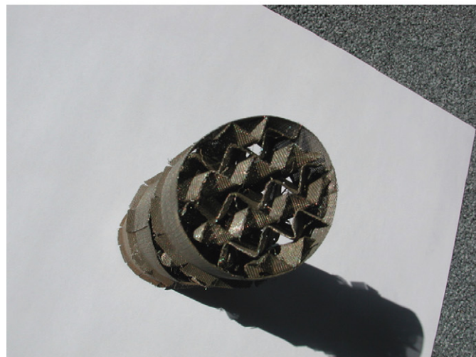
Fig. 2. Pictures of the structured packing Sulzer EX ® .
