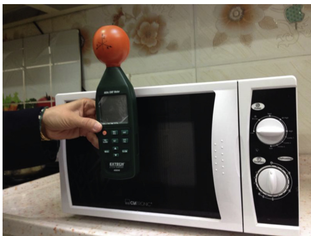
Fig. 1 – GHP meter used to measure the power intensity, electric and magnetic fields in some House.
