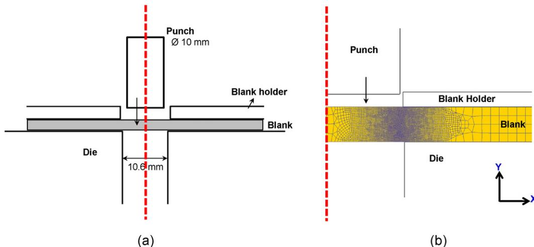
Fig. 1. (a) Schematic diagram for the punching process and (b) initial finite element mesh for FEA of the punching process.
