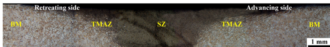
Fig. 2. The cross sectional macrostructure of the joint.
