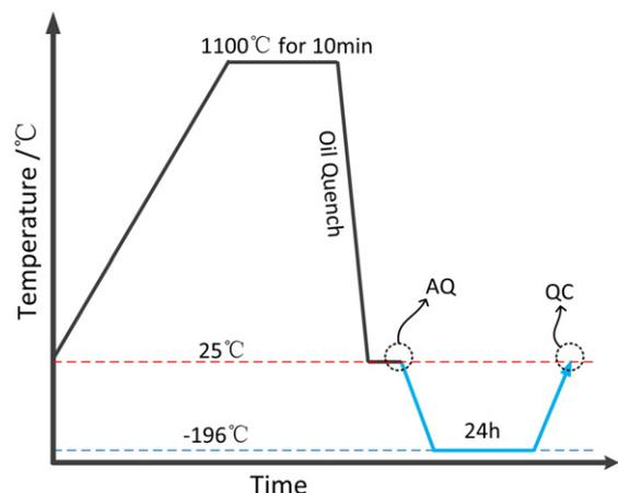
Fig. 2. Schematic AQ and QC heat treatment schedules for the investigated steel.
