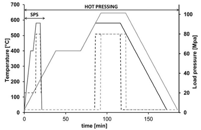
Fig. 2. HP and SPS sintering cycles; the temperature is in continuous lines, the pressure in dotted lines.
