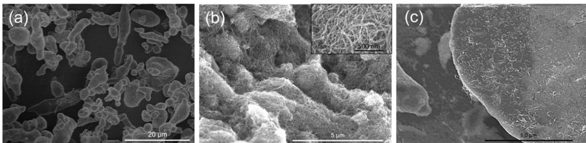
Fig. 1. (a) Raw aluminum powder, (b) CNT and (c) CNT/Al composite powder used to prepare the composite materials.
