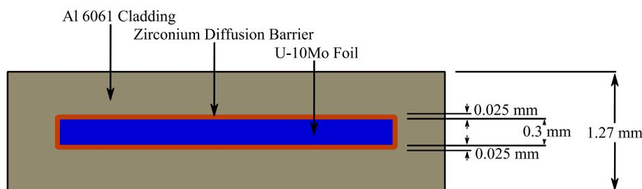
Fig. 1. Cross section of a monolithic U–Mo fuel plate.
