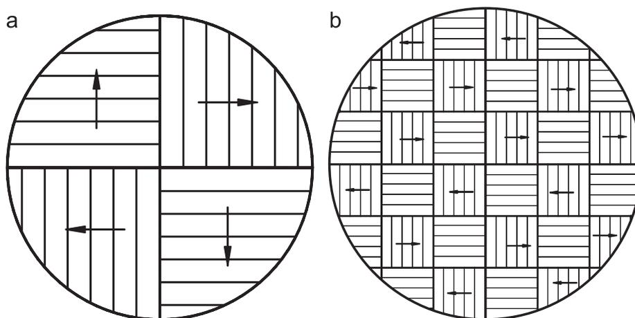
Fig. 2. Single-turn and multi-turn louver-baffle plates. (a) Single-turn louver-baffle plate, and (b) multiple-turn louver-baffle plate.
