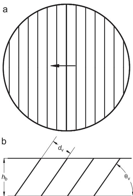
Fig. 1. Schematic of louver baffles. (a) Top view, and (b) sectional view (part).
