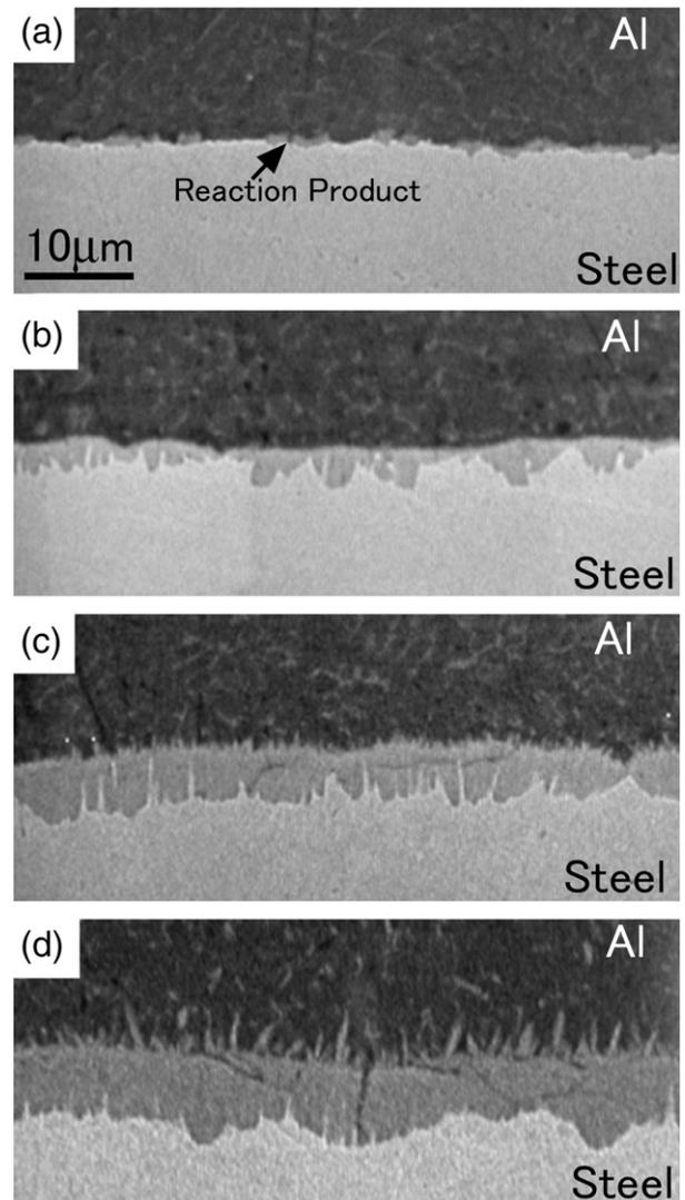
Fig. 3 – SEM images of the weld cross-section at the Al/steel interface; (a), (b), (c) and (d) taken from the positions (A), (B), (C) and (D) in figure 2, respectively.
