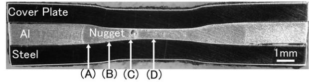
Fig. 2 – Optical micrograph of the weld cross-section.
