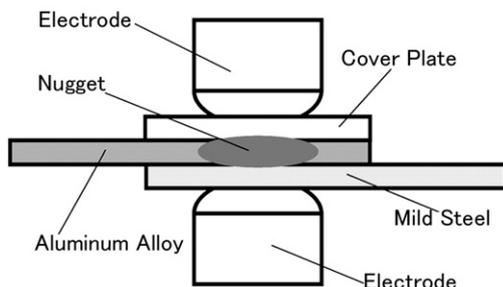
Fig. 1 – Schematic diagram of resistance spot welding with cover plate.
