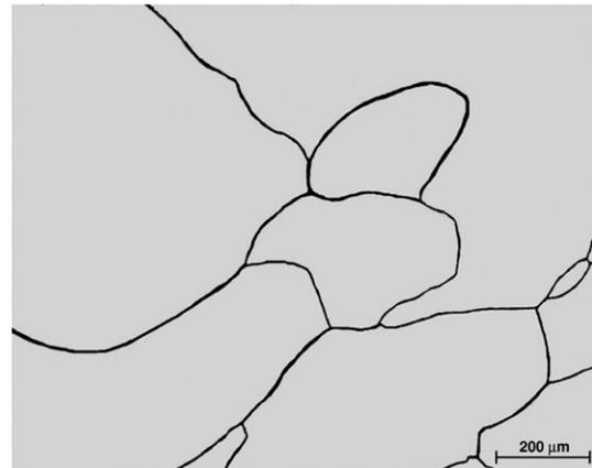
Fig. 3 – Optical micrographs of the Fe-40 at.% Cr alloy solution treated and subsequently aged at 500 °C for 750 h.
