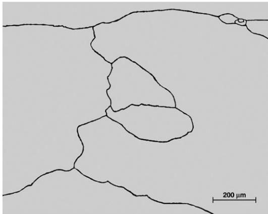
Fig. 1 – Optical micrographs of the as-cast Fe-40 at.% Cr alloy.
