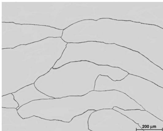
Fig. 2 – Optical micrographs of the solution treated Fe-40 at.% Cr alloy.
