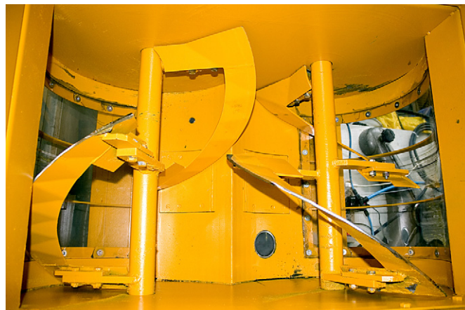
Fig. 1. View of the mixing chamber of the twin-shaft-paddle laboratory mixer with spiral mixing tool.
