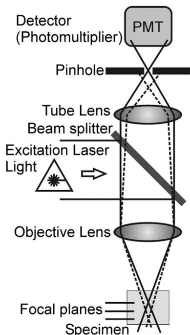
**Fig. 1 – Schematic diagram of the optical pathway in a laser scanning confocal microscope.**
