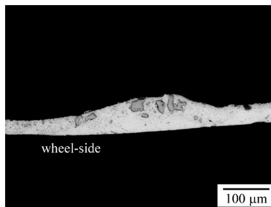
Fig. 4–Microstructure of a melt-spun ribbon (orifice diameter 1.8 mm) with numerous unmelted particles. (LM, alloy \text{Al}_{92}\text{Mn}_3\text{Be}_5 ).
