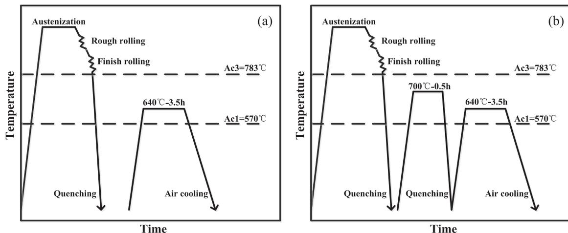
Fig. 1. Schematic diagram of the hot rolling and intercritical annealing process: (a) IA640; (b) IA700-640.
