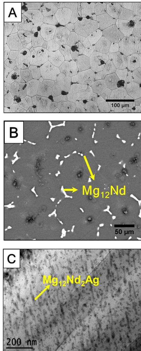
Fig. 1. Microstructure of an as-received cast QE22 magnesium alloy. (A) Optical micrograph showing equiaxed microstructure (B) Back scattered electron (BSE) micrograph; arrow indicates the  $\text{Mg}_{12}\text{Nd}$  eutectic (C) TEM micrograph showing  $\text{Mg}_{12}\text{Nd}_2\text{Ag}$  precipitates.
