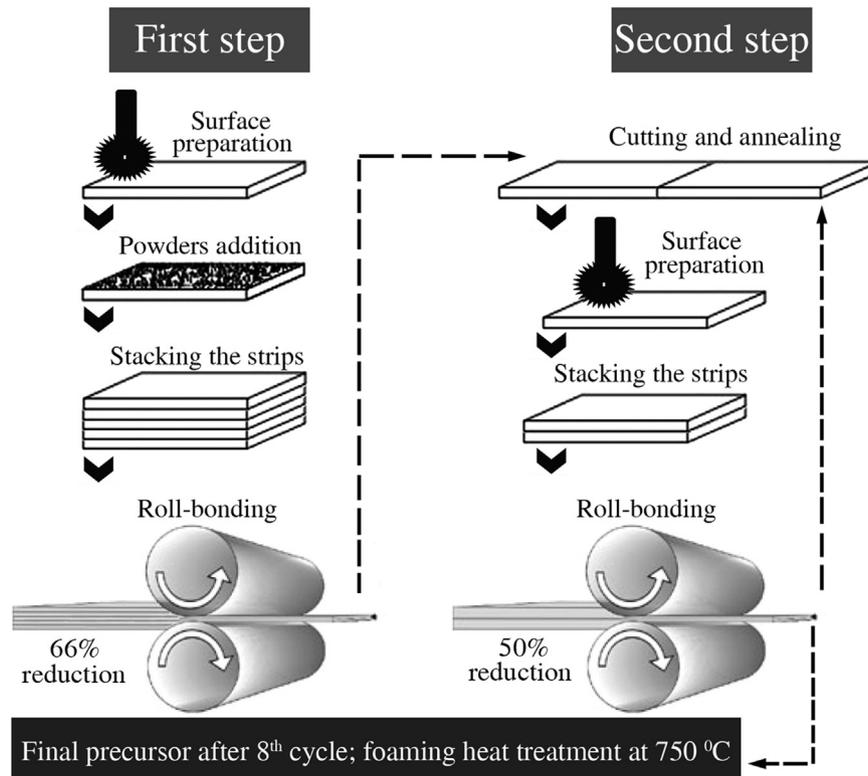
Fig. 2. Schematic illustration of foam manufacturing via CAR process.
