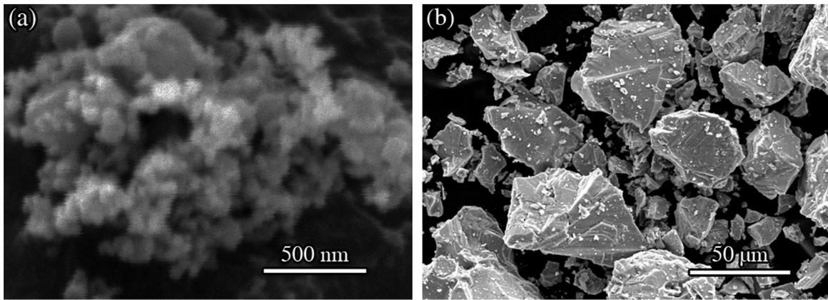
Fig. 1. SEM micrographs of (a) nano-SiC, and (b) micro-TiH<sub>2</sub> particles.
