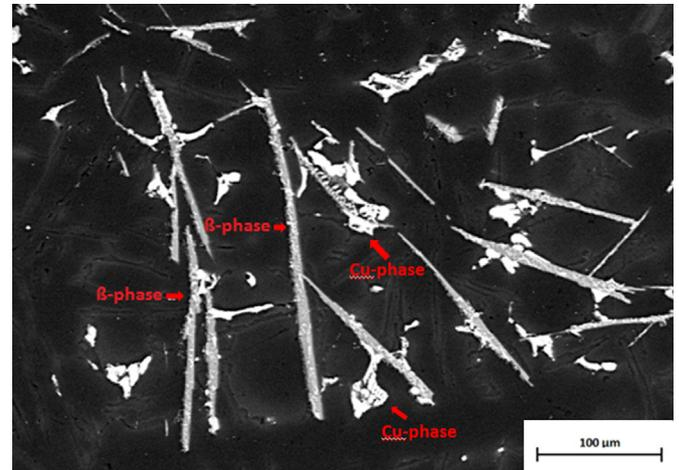
**Fig. 2.** Long needle-like  $\beta$ -phases with Cu-rich intermetallics.
