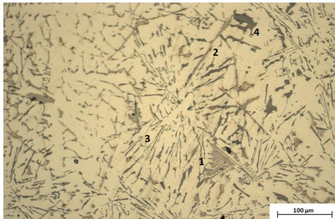
**Fig. 1.** Main inclusions of recycled Al-Si-Cu alloy: 1 –  $\alpha$ -Al<sub>15</sub>(FeMn)<sub>3</sub>Si<sub>2</sub>, 2 –  $\beta$ -Al<sub>5</sub>FeSi, 3 – Eutectic silicon, 4 – CuAl<sub>2</sub>.
