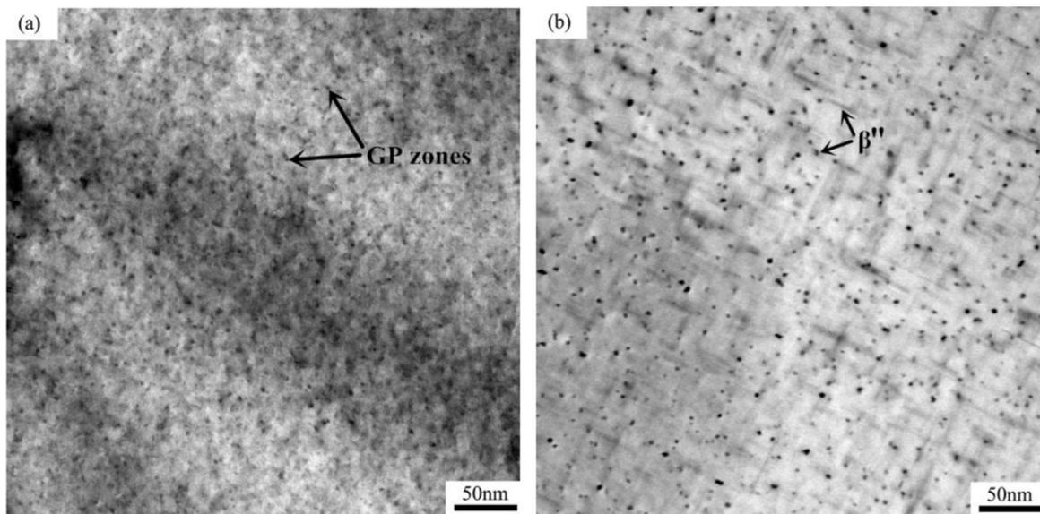
Fig. 1. TEM bright-field images of 6016 Al alloys under (a) PA and (b) T6 condition.
