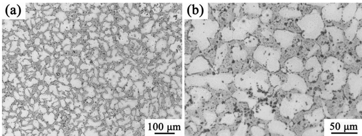
**Fig. 3.** Optical microstructure of the as-cast LAZ832–0.5Y alloy.
