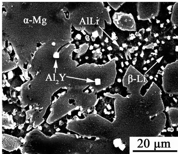
**Fig. 2.** SEM image of the as-cast LAZ832–0.5Y alloy.
