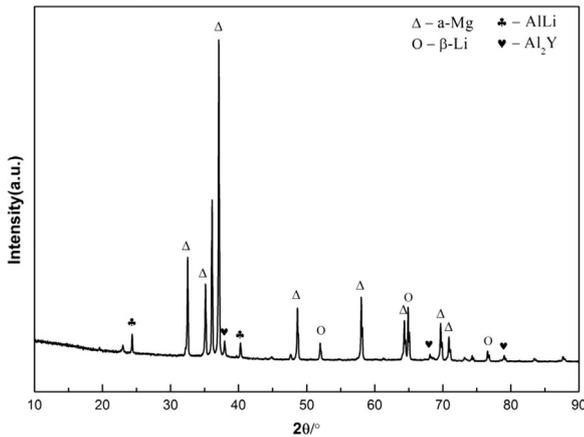
**Fig. 1.** XRD pattern of the as-cast LAZ832–0.5Y alloy.
